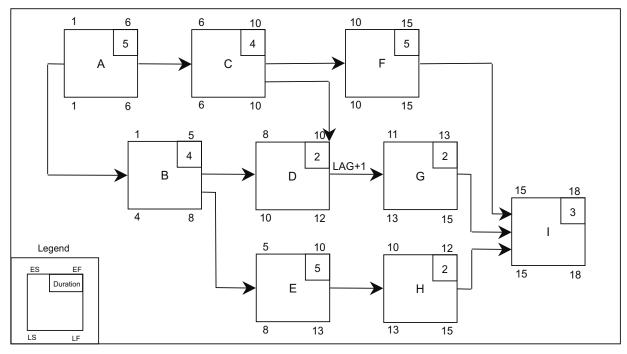
Figure 6-10. PDM Example with Lag Time
