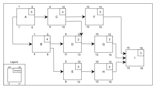
Figure 6-9. PDM Example—Early and Late Start and Finish Times
