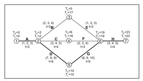
Figure 6-6. PERT Example with Slack Time
