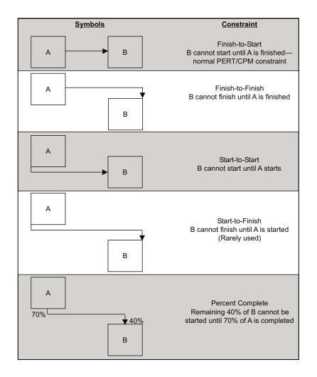
Figure 6-2. Example PDM Relationships/Constraints
