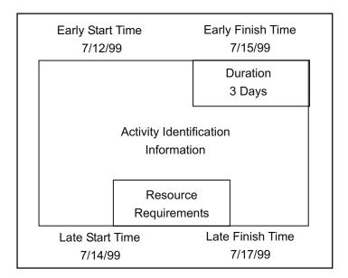
Figure 6-4. Example PDM Activity Node
