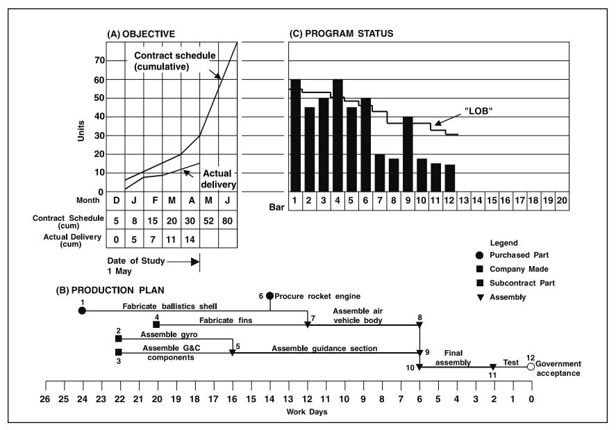
Figure 7-1. Line of Balance Technique
