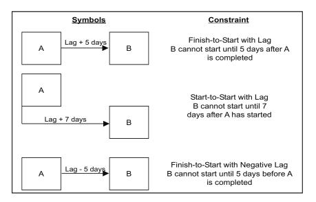
Figure 6-3. Example PDM Constraints with Lag Time
