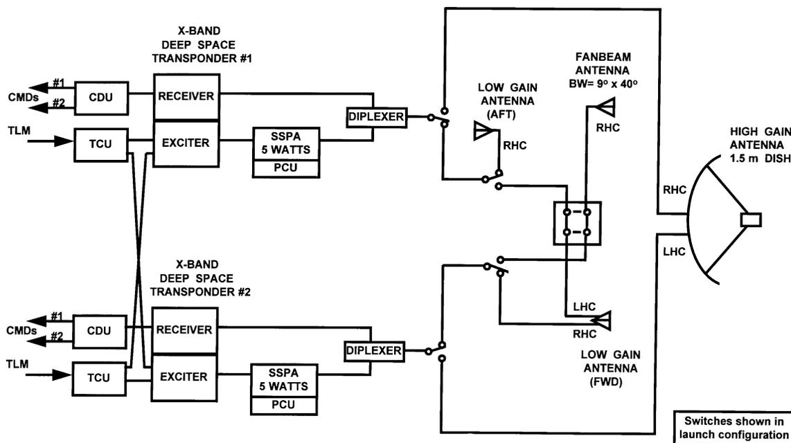
Fig. 7. Telecommunication Block Diagram
