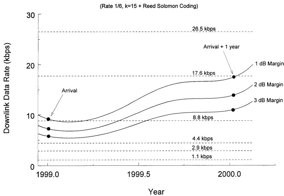
Fig. 8. Downlink Data Rate at Eros with DSN 34m Antenna
