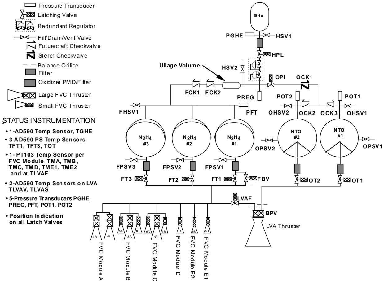
**Fig. 6. Propulsion System Hydraulic Schematic**
