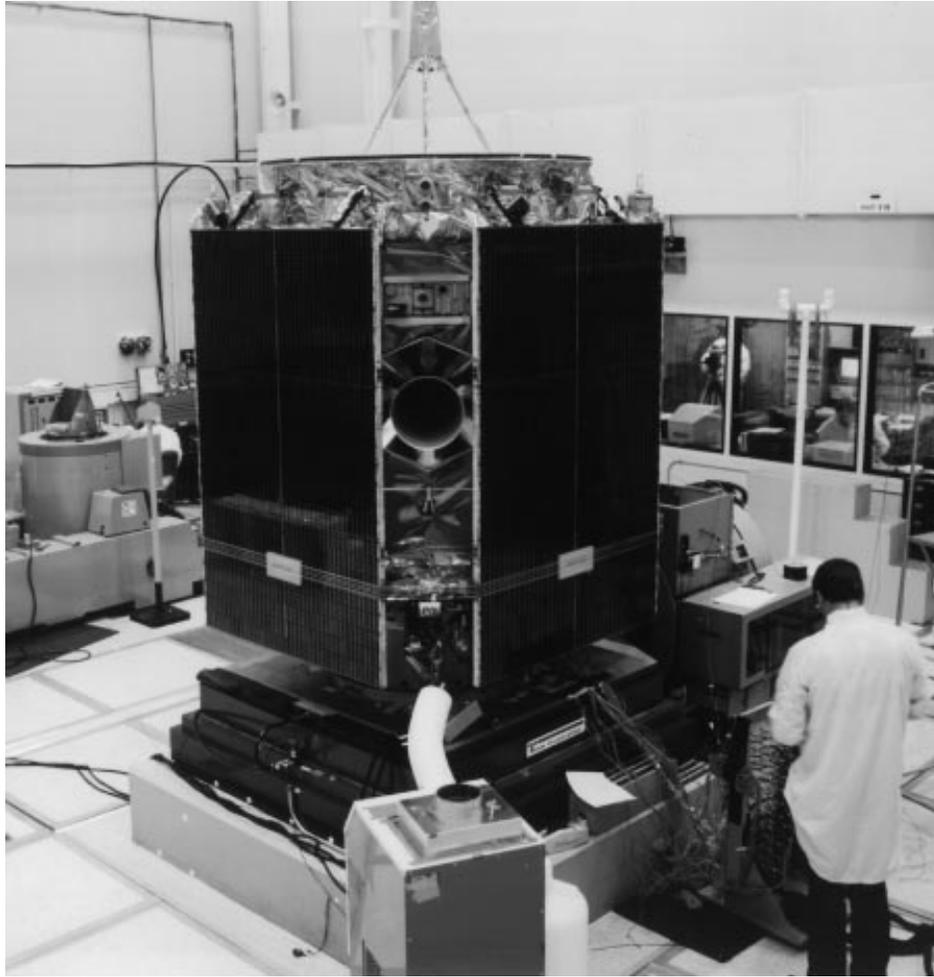
**Fig. 3. Spacecraft in Launch Configuration During Vibration Testing**
