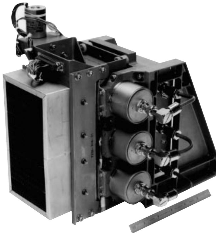
**Fig. 12. X-ray Spectrometer**
