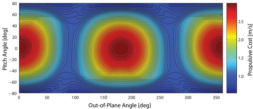
Figure 8.6: Optimal  $\Delta V$  with respect to separation conditions between two objects.[3]
