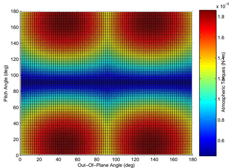
Figure 8.7: The atmospheric drag torque with respect to the attitude of the satellite.
