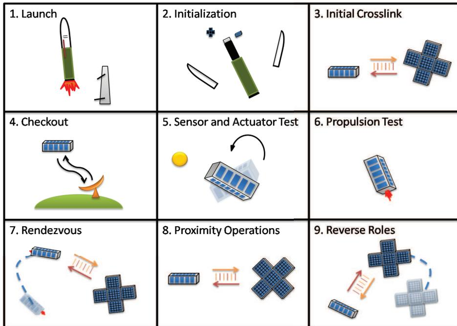
Figure 5.1: Pictorial Concept of Nominal Operations for the Paradox Mission.
