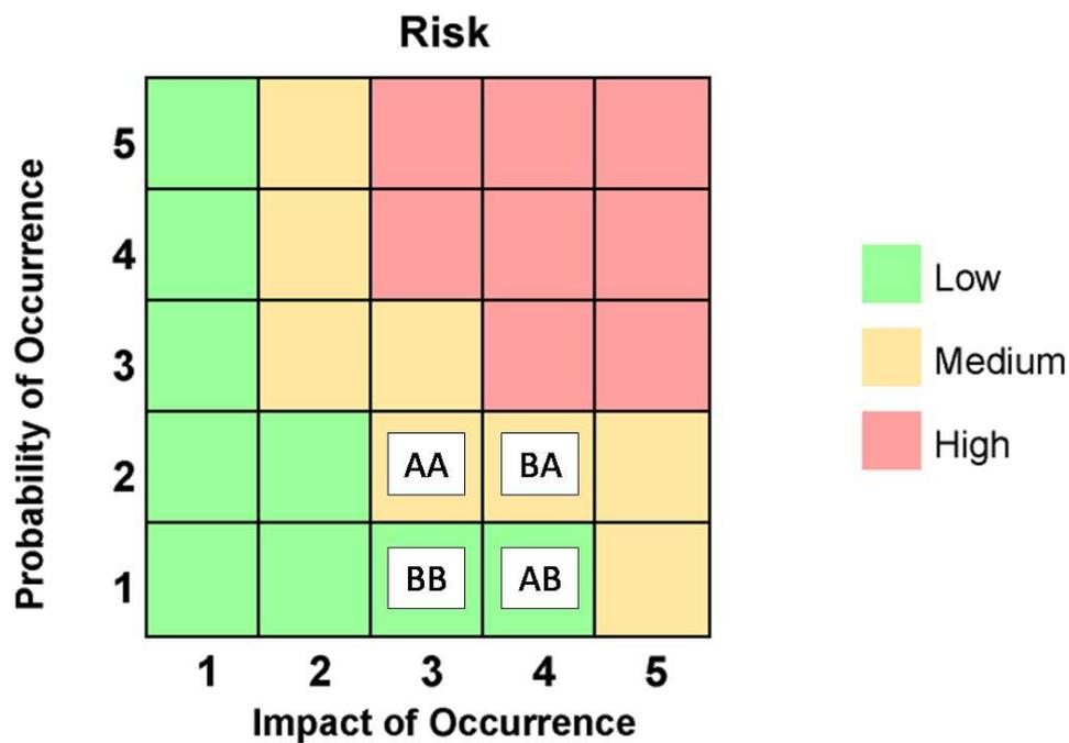
Figure 10.2: Risk matrix used to communicate risks from FMEA on rendezvous guidance algorithm.
