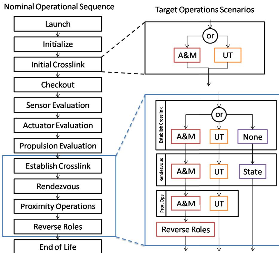
Figure 5.2: General concept of operations indicating the three different mission scenarios for the Paradox mission.
