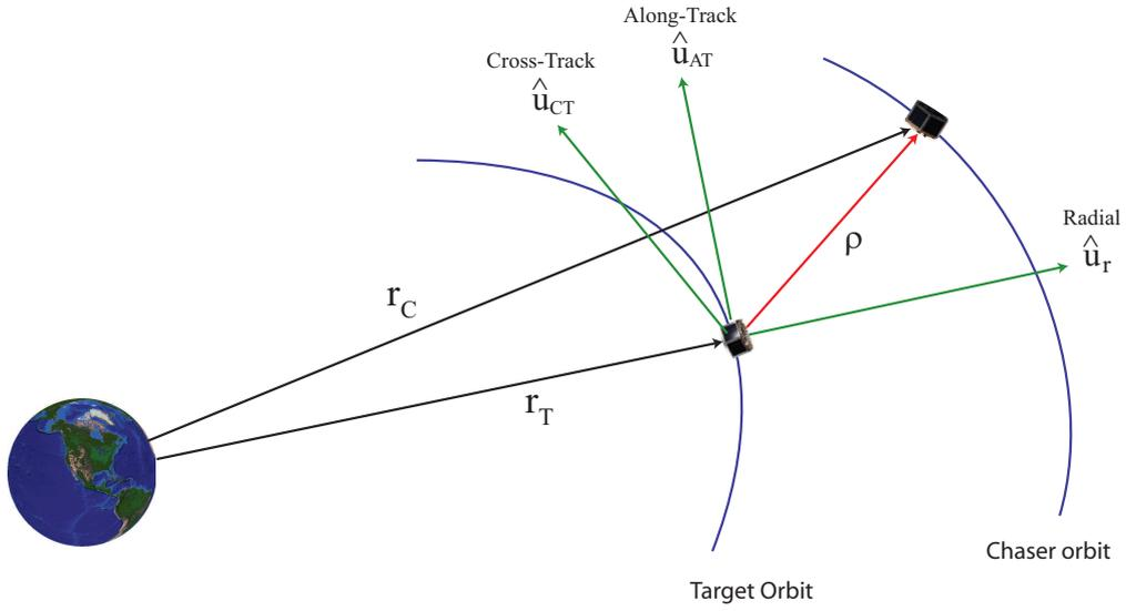
Figure A.1: Description of positioning in relative reference frame.[3]
