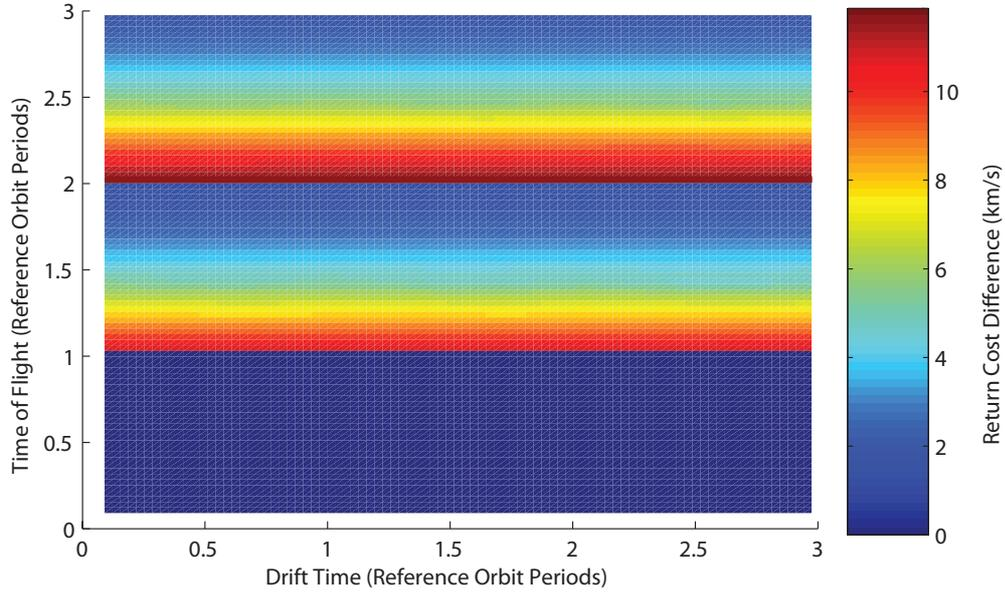
Figure 8.3: Difference between  $\Delta V_L$  and  $\Delta V_{CW}$  with respect to drift and transfer times.
