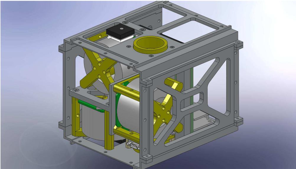
Figure 8.12: A custom configuration of three SI-30 mounted in a custom satellite structure.
