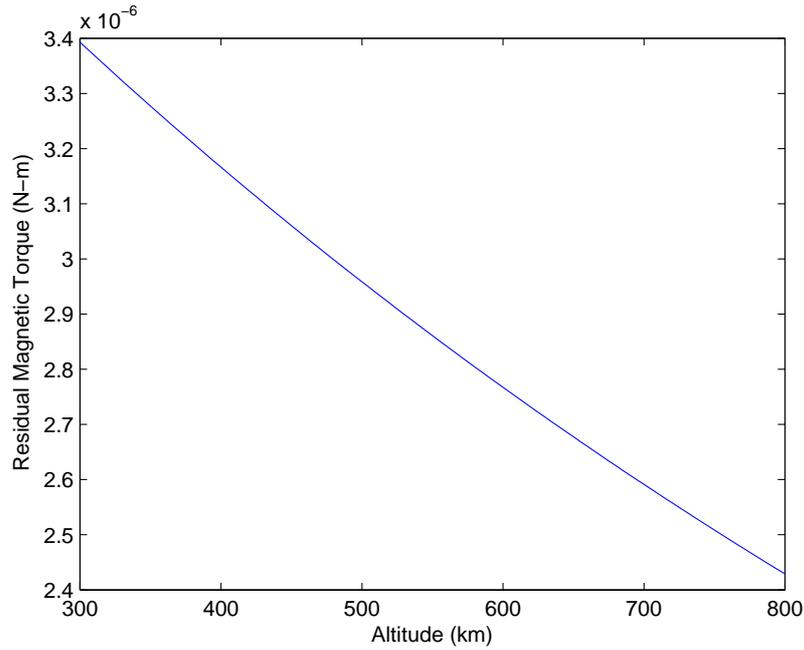
Figure 8.9: The residual magnetic dipole torque with respect to altitude given the worst case attitude.
