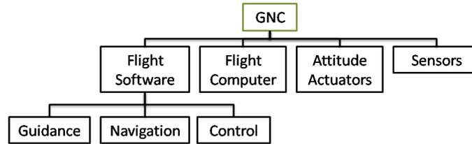
Figure 6.2: GNC subsystem hierarchy for the Paradox Mission.
