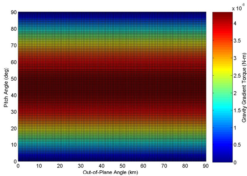
Figure 8.10: The gravity gradient torque with respect to the attitude of the satellite.
