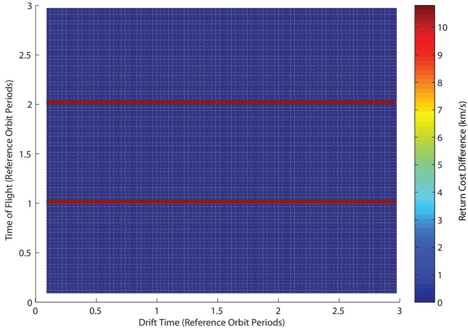
Figure 8.4: Difference between the  $\Delta V_L$  and  $\Delta V_{CW}$  with respect to drift and transfer times.
