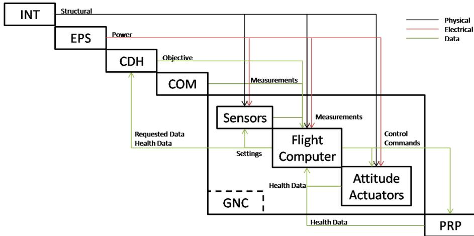
Figure 6.4: Basic interface definition for the GNC subsystem with respect to every other subsystem.
