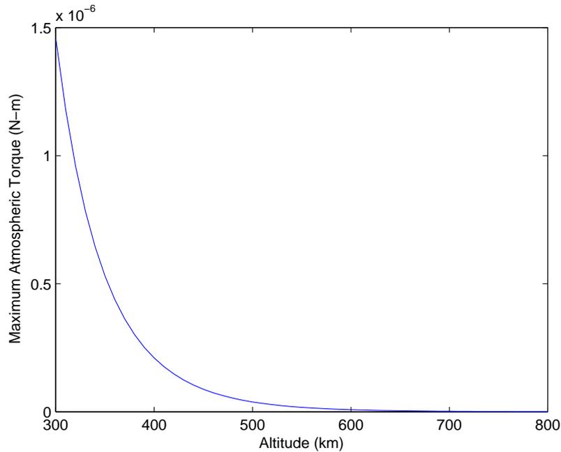
Figure 8.8: The atmospheric drag torque with respect to altitude given the worst case attitude.
