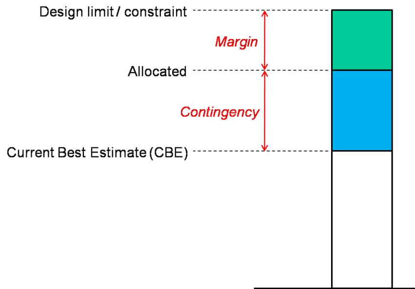
Figure 9.1: Margin and contingency with respect to any resource constraint.
