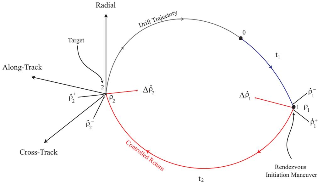
Figure 8.1: Description of drift and return trajectories in the relative reference frame.[3]
