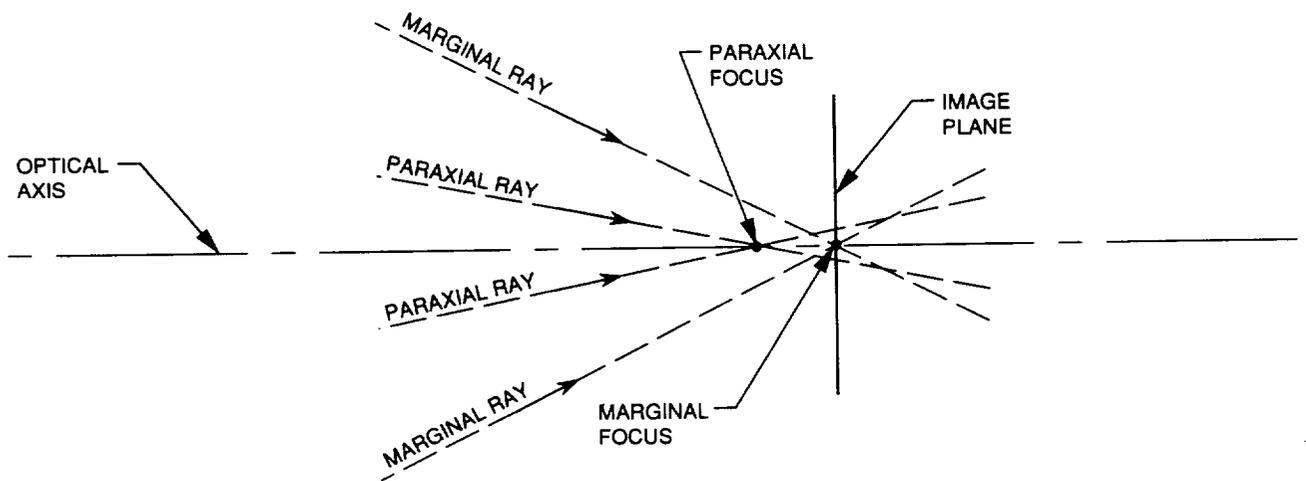
**Figure C-4. Image-plane enlargement of the HST Ritchey-Chretien optical system. In the HST, too much material from the edges of the primary mirror was removed, and the marginal focus was moved past the paraxial focus. This is characteristic of an optical system overcorrected for spherical aberration.**
