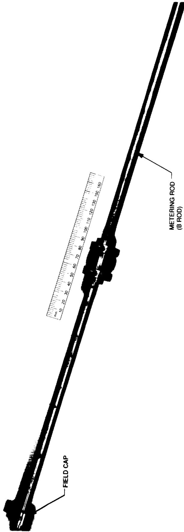
Figure 7-2. Metering rod (B rod) used to space the field lens and the center of curvature of the lower mirror in the reflective null corrector.
