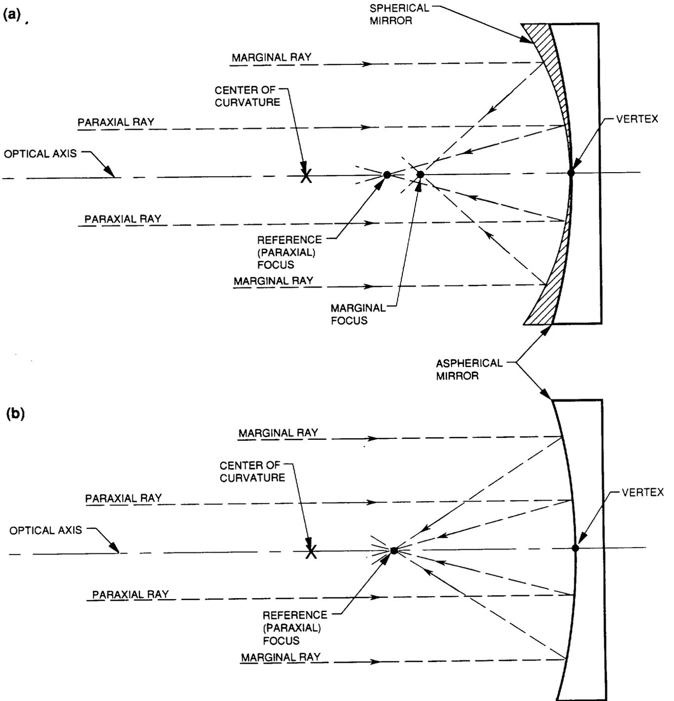
**Figure C-1. Light-path comparison between spheric and aspheric mirrors. (a) The perfectly spherical mirror shows light reflecting to the two extreme foci, causing spherical aberration. (b) To remove this spherical aberration, an aspheric mirror is created by grinding down the edges of the mirror.**
