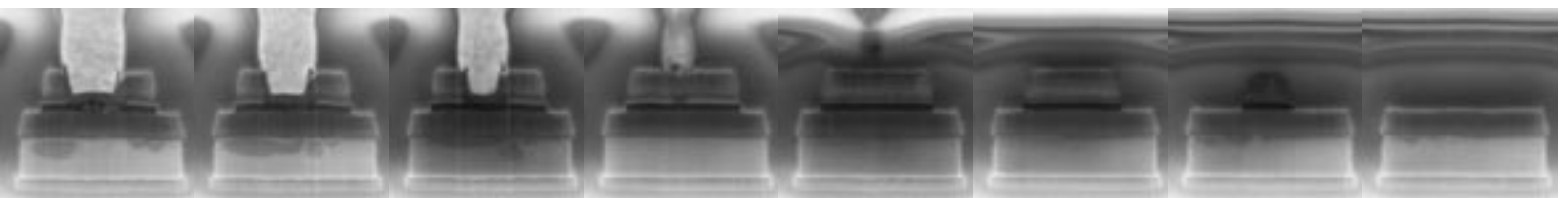
Multiple 3-D solid-model reconstructions of an FPGA antifuse. The model can be sliced along X, Y, and Z planes to visualize more detailed information with respect to the chemical composition of the interior geometries.
