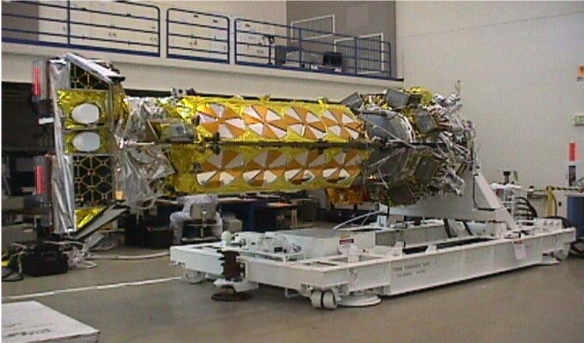
Figure 5-2: NOAA N Spacecraft in Horizontal Position on TOC
