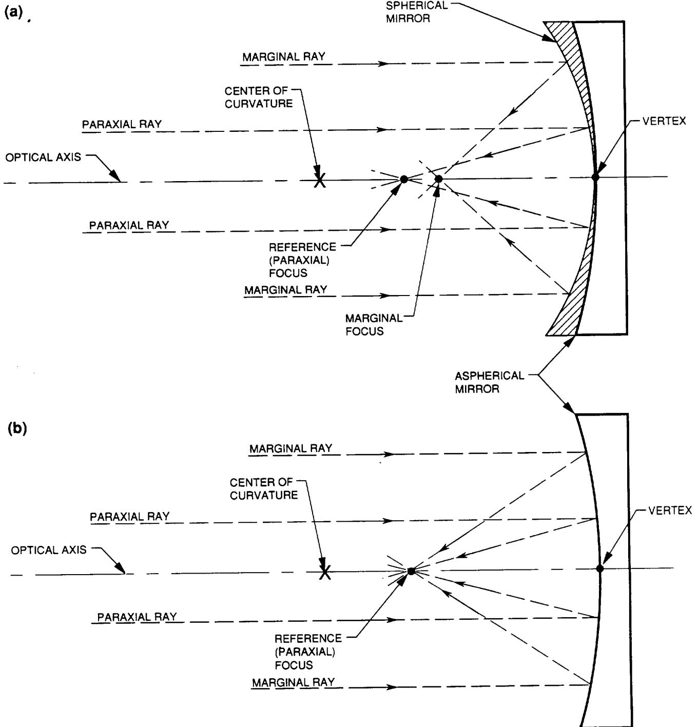
**Figure C-1. Light-path comparison between spheric and aspheric mirrors.**
